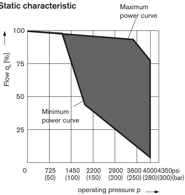
The power characteristic is set at the factory, please state your requirements in clear text e.g. 27 HP (20 kW) at 1800 rpm.
