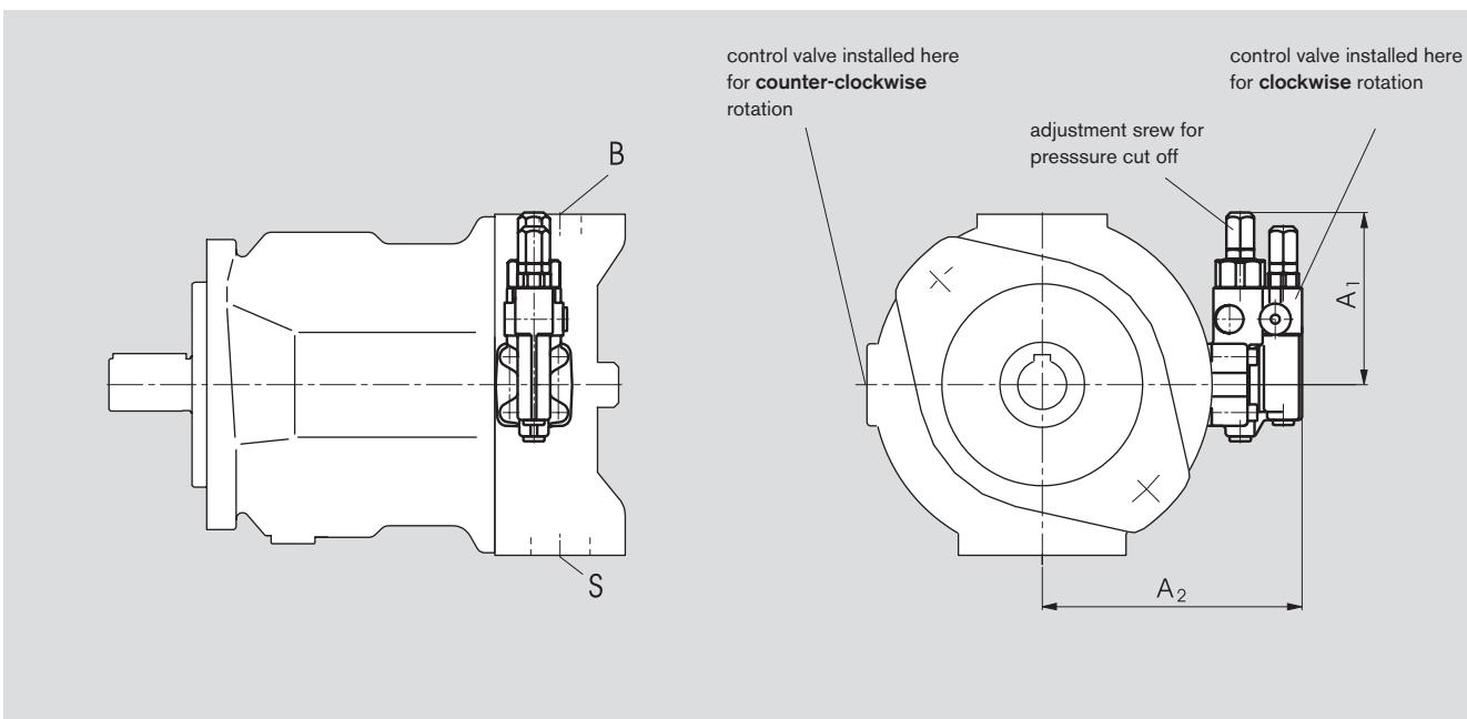
On sizes 18 to 100 the DFR valve is used. The flow control spool is blocked and not tested.
