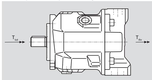
The drive torques for pump 1 and pump 2 can be split up as required. However the max. permissible input torque  $T_{tot}$  as well as the max. permissible through drive torque  $T_{thr}$  may not be exceeded.
