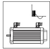
Duty type: Short time operation S2 with terminal box connection
