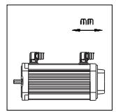
**Asynchronous servo motors MDFQA 100...132, mounting position B35**
