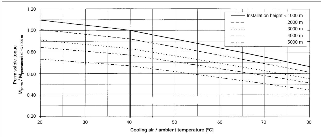
Asynchronous servo motors MDXKA and MDFQA, for motors with separate fan MDFKA and MDFQA
