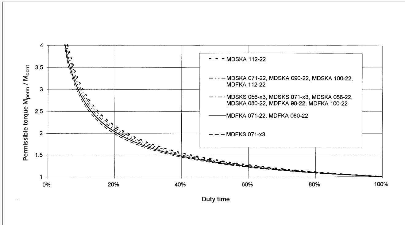
Duty type: Continuous operation S6, 1 min load cycle with terminal box connection
