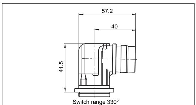
Encoder plug (resolver / Sin-Cos / incremental encoder)
